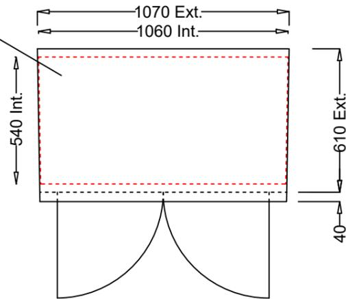
1No. 870 x 1080 mm, 18mm Surface Treated Ply Backboard
